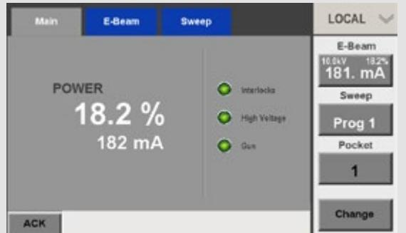
One universal remote controller provides access to all operation functions.
