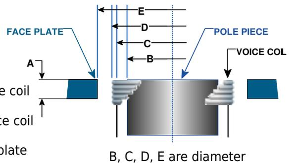
The recommended tolerance on ferrofluid quantity is  $\pm 10\%$  which is best maintained through the use of a positive volume displacement dispenser. Maintaining the proper ferrofluid quantity is critical as overfilling the gap is wasteful and can lead to leakage while underfilling the gap minimizes the heat transfer benefits of the ferrofluid, compromises the fluid's long term reliability and can lead to response anomalies in the loudspeaker.
