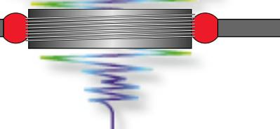
There are three important physical properties of ferrofluid that must be understood to successfully design fluid-filled audio speakers and select the best fluid: saturation magnetization, viscosity and volatility.
