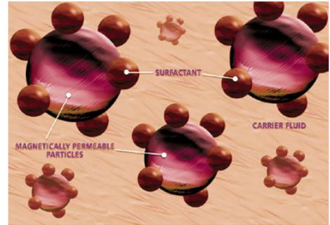
When a magnetic field is applied to a ferrofluid, the magnetic moments of the particles orient along the field lines almost instantly. The magnetization of the ferrofluid responds immediately to the changes in the applied magnetic field and when the applied field is removed, the moments randomize quickly.
